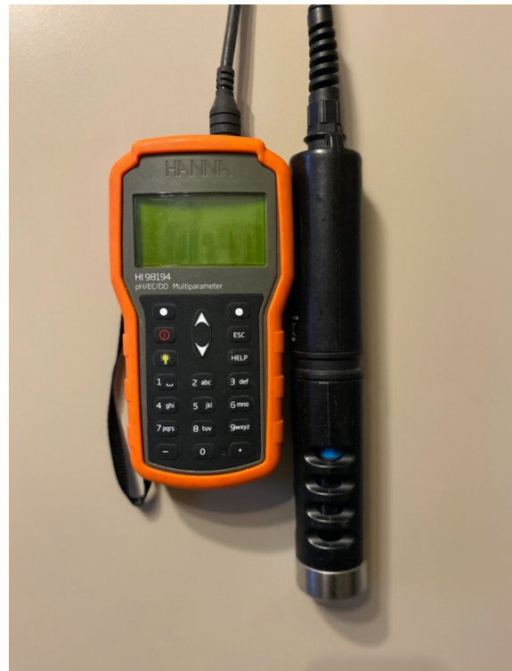
Photo 20: the Hanna Meter is used to assess water quality
